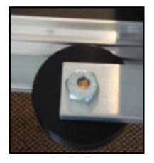
☐ The adjusting cams for the carriage are located on the front carriage axle. It is crucial that these wheels are set properly for the smoothest operation. When you adjust the front carriage wheels, you are also adjusting the back wheels at the same time.
