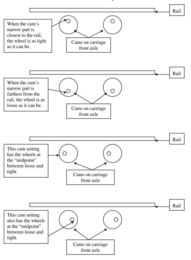
You can set the "feel" of your carriage by making the wheels looser or tighter. If the machine feels tight when moving it left to right, loosen the wheels slightly, but set each cam to the same position. If the machine feels loose or sloppy, tighten the wheels slightly. Use the illustrations above for reference.
