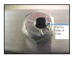
Wheel adjustment is accomplished by rotating the carriage wheel adjustment cams into the correct position. Remember, these cams are located on the front carriage axle.
